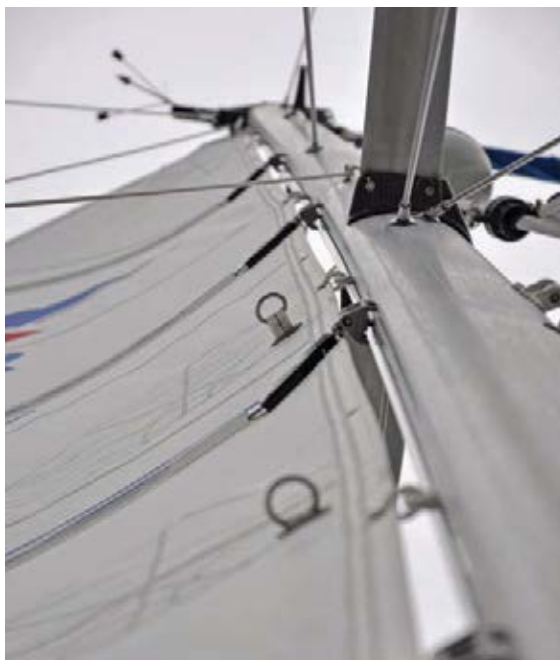
Below: Fully battened sail cars had to be adapted to fit the old Selden mast track
